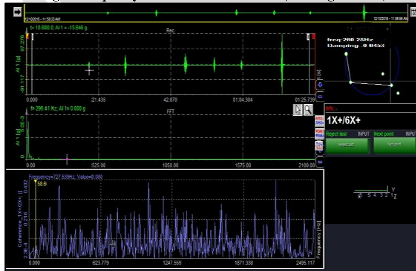
Fig-8: Frequency is 260.28 Hz for Mode 2 (Modified Muffler)
