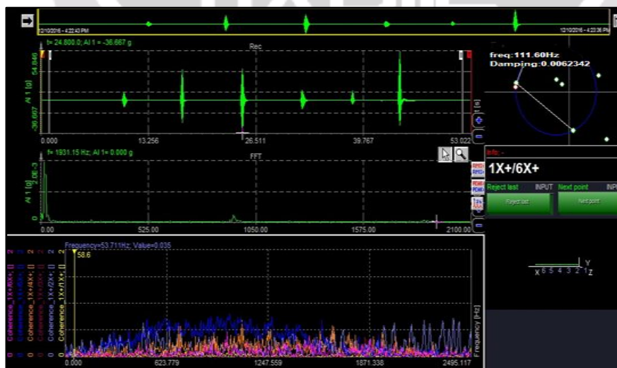
Fig-5: Frequency is 111.60 Hz for Mode 1(Existing Muffler)
