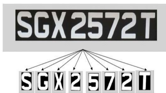
Fig. 11. Example of Plate Segmentation.
