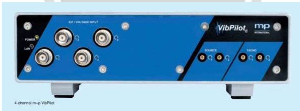
Fig-5: Dynamic Signal Analyzer
