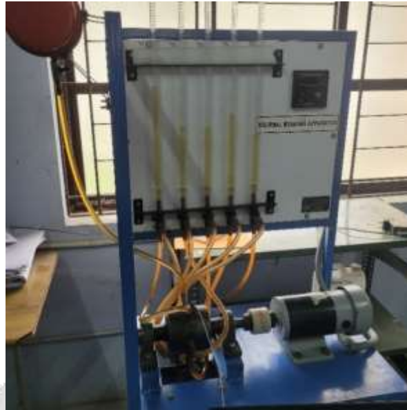
Fig-1: Journal Bearing Apparatus
