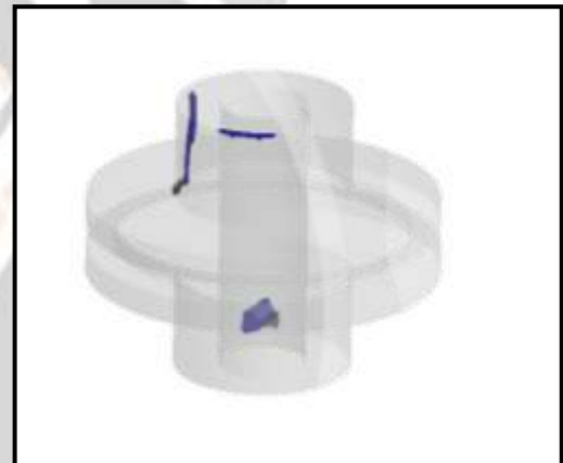
Figure -8 : the simulation results showing the number of air traps for the flow of 3 m/s
