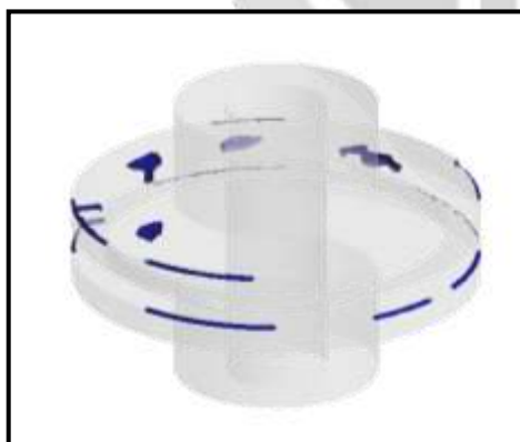
Figure -3: the simulation results showing the number of air traps for the flow of 0.5 m/s
