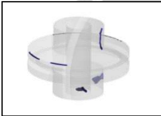
Figure -7 : the simulation results showing the number of air traps for the flow of 2.5 m/s
