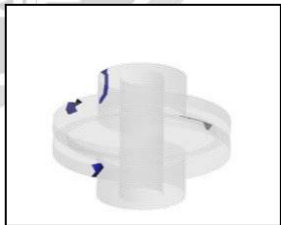
Figure -10: the simulation results showing the number of air traps for the flow of 4 m/s
