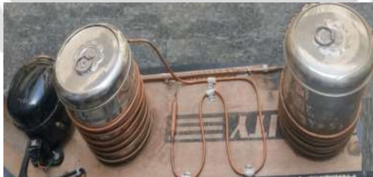
Fig.3 Experimental Setup of Modified VCR Cycle
