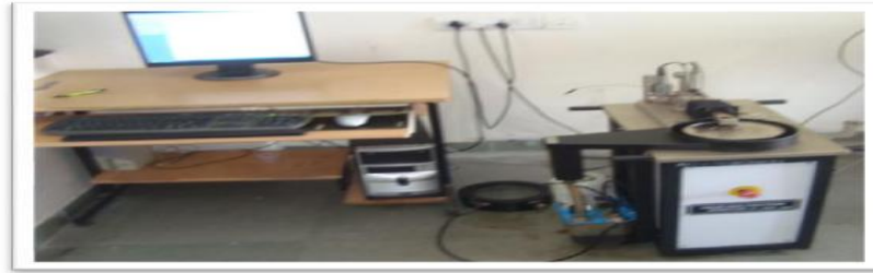
Fig 01: Experimental Set Up of Pin on Disc Tribometer
