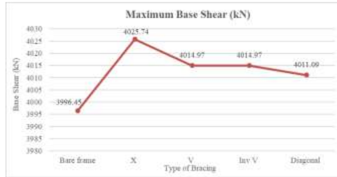
Chart -3: Graph of Maximum Base Shear vs Type of bracing
