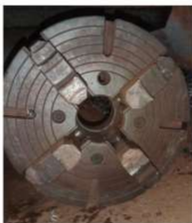
Fig -10: 4-jaw Independent Jaw Chuck
