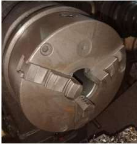
Fig -9: 3-Jaw Self Centering Chuck
