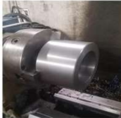
Fig -10: Inverted 3-jaws Workholding
