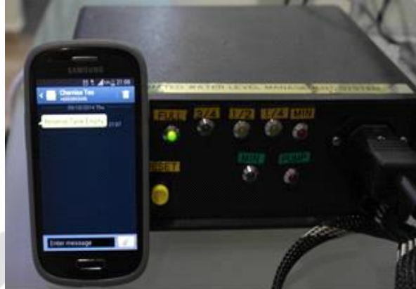
Figure 11: SMS alert sent to user when reserve tank level is below the minimum level.
