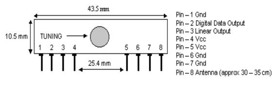
Frequency: 433.92MHz Modulation: AM Operating Voltage: 4.5 - 5.5 VDC Output: Digital & Linear
