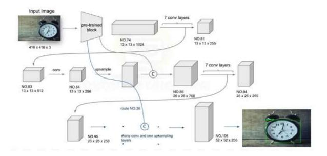
Fig-1: Architecture of yolov3
