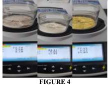
Figure 4 - Represents color of the powders, done in colorimeter Finger millet  $-L^*=71.74$ ,  $a^*=3.68$ ,  $b^*=9.18$
