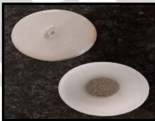
Figure 3.1.2 Sample turned into ash after keeping in muffle furnace
