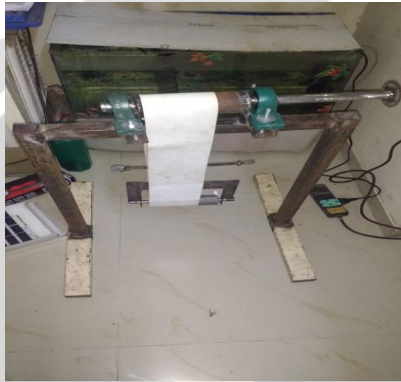
Fig5.1. -Actual construction of oil skimmer.
