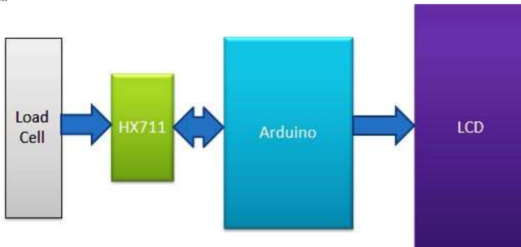
Fig no 5 Working of load cell flow chart
