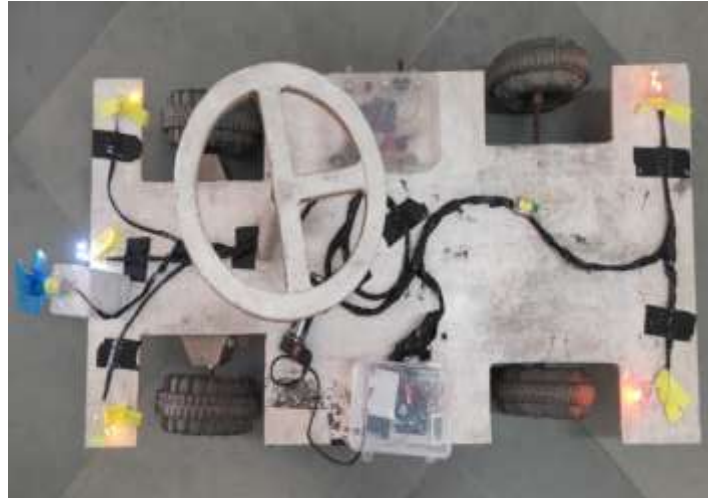
Fig (c): Implemented prototype of EV Battery management System
