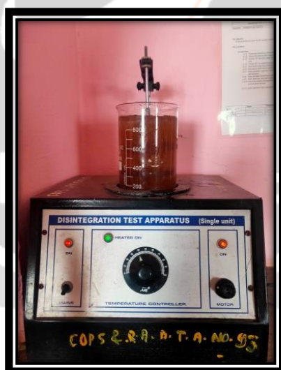
Fig 6. Disintigration Test Appratus
