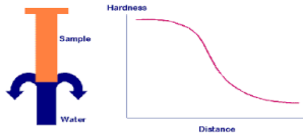
Fig. 5.1. jominy graph and test apparatus.
