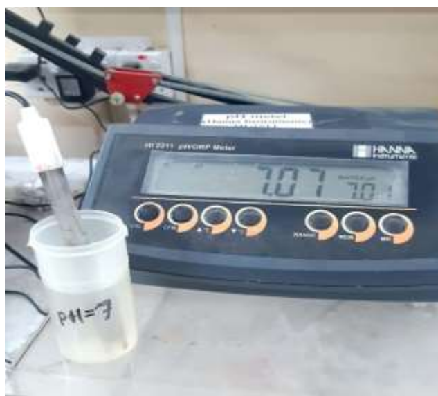
Figure-1: Measurement of pH level of Buffer Solution to check the validity of pH Meter
