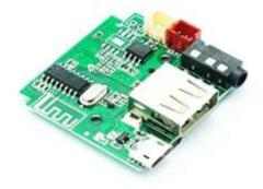
2. <u>SPEAKER</u>: Speaker output power is determined by  $V_{CC}$  (supply voltage) and the speaker load (in ohms). 20W output results from a supply voltage of 18V and a speaker load of 8 $\Omega$ . For 10W output the conditions are: 13V  $V_{CC}$  and 8 $\Omega$  speaker load.
