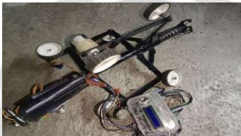
Fig 11. Internal Pipe Inspection Robot
